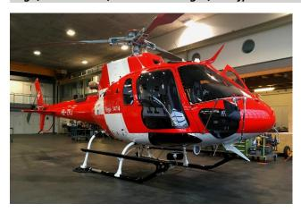
A solution like the MPVK for the AS350 / H125 was long overdue. The Maximum Pilot View Kit means to us, that we train pilots much faster and safer to a high level regarding HESLO and HEC operation. The widest possible field of vision is crucial for every pilot to ensure safety in the daily operation; the ultimate target of Rega. Congratulations to the SRS team for their impeccable work, we are highly satisfied!
